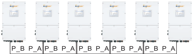
Figure 3.24 Parallel Terminal Connection
