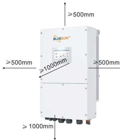
Figure 3.5 Inverter Mounting Clearances
